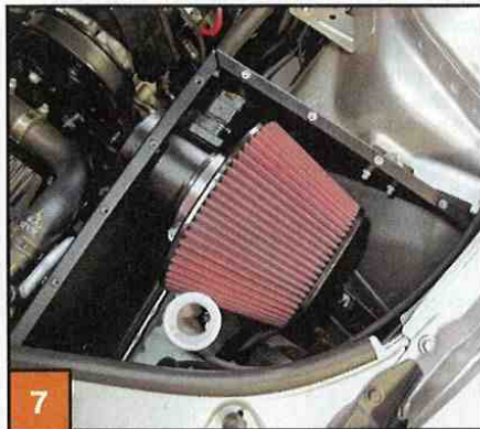
▲ Next, we installed the ADM conical filter and reconnected the MAF sensor. The larger filter and sealed airbox are keys to making more power. After all, the last place you want hot engine bay air is around your filter.
