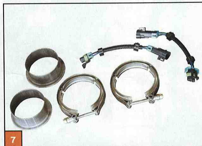
▲ Included with the JBA headers and cats are all the parts needed to mate the long tubes to either a stock exhaust system or, as in our case, their aftermarket cat-back system. Also in the box are extension harnesses for the forward two O2 sensors along with bolts and gaskets.
