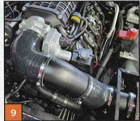
▲ And here's the fully assembled intake tube. The system utilizes 4-inch (100mm) ID tubing from the filter to the throttle body.
