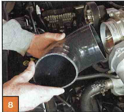
▲ We then assembled the air intake tubing, starting with the silicone hose off of the throttle body.
