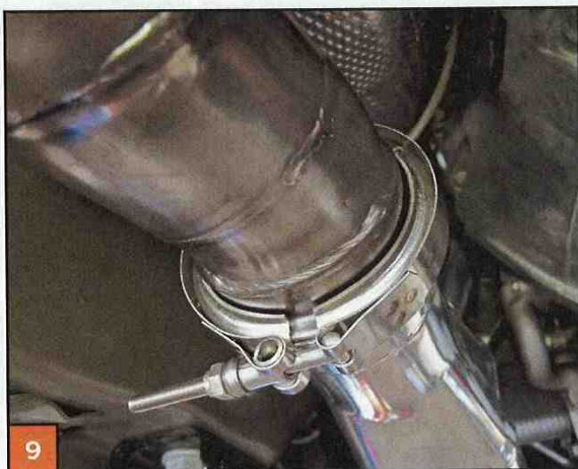
▲ Using the stainless band clamps, we attached the new JBA high-flow cats to the long tube headers.
