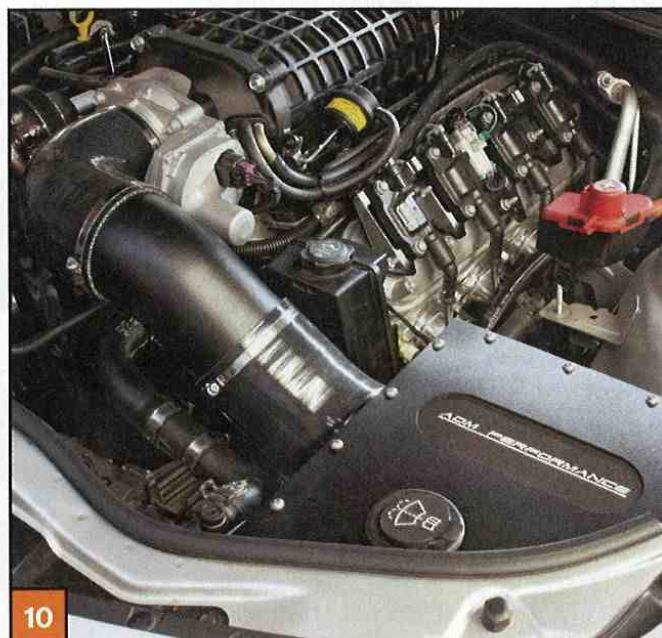
▲ Lastly, we installed the airbox lid. As you can see, the inlet for the washer bottle comes through the lid, which is why we needed to loosen it up first. Once the lid was in place, we snugged up the washer bottle bolts and refastened the inner fender. It looks
