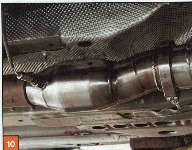
▲ The rears of the JBA cats were then secured to the rest of the exhaust system using the factory band clamps. We then re-
